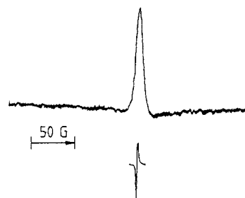
Figure 4. X-band EPR spectrum of bulk sodium showing the highly asymmetric derivative line shape. Microwave power 10 mW, modulation 5 G, gain 3.2 \times 10^2 ; g (corrected for line shape) = 2.0014 \pm 0.0002 , \Delta H_{pp} = 17 \pm 1 G.
